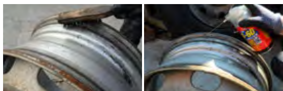
<Retirez la corrosion>
